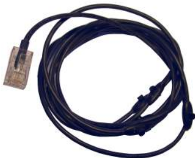
T-String (TS) cable with 6 x DS18B20 temperature sensors.
